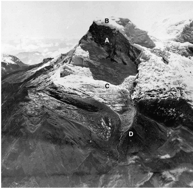
Fig. 4. Pre-1962 oblique aerial photograph of the North Peak of Huascarán. View is to the east. Both the 1962 and 1970 mass movements originated as falls from the steep west face (A). Bedrock is massively jointed granodiorite. Note the summit glacier ice-cap (B). In both events, the fragmenting mass traveled over the steeply sloping surface of Glacier 511 (C) and was channeled by the Little Ice Age terminal moraine complex (D). We hypothesize that the steep west face is the scarp of the massive pre-Columbian rock avalanche, the deposits of which cover the slopes below Huascarán and fill the Rio Santa valley. (photograph: Servicio Aerofotográfico Nacional de Perú 11371; August 16, 1948).
