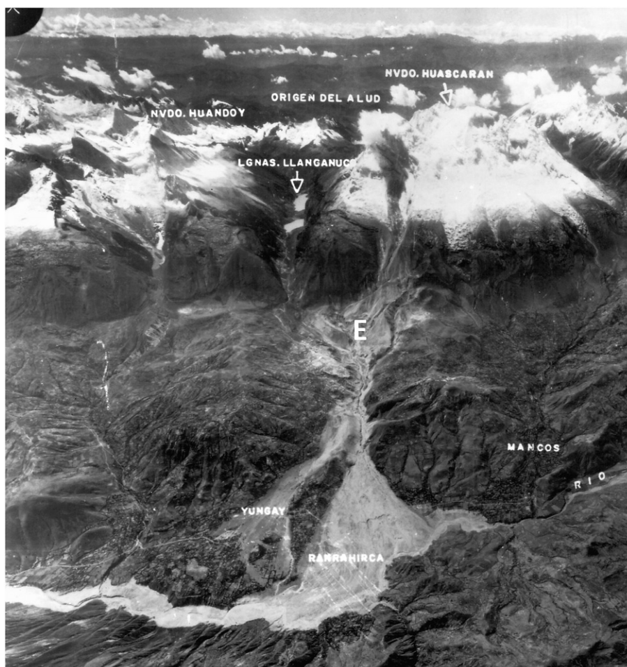
Fig. 1. Oblique aerial view to the east of the May 31, 1970 Huascarán event showing source, path, devastation of Yungay and the Ranrahirca fan, and beginning of downstream distal debris flow/debris flood following the Rio Santa off to the left. The extensive area of entrainment is seen below the terminal moraine system of Glacier 511 (E). Also visible is the peak of Huascarán, the source of an ice/rock fall triggered by the 1725 earthquake which generated a debris flow that led to the destruction of the town of Ancash. (Photograph and annotation; Servicio Aerofotografico Nacional de Perú; June 13, 1970).
